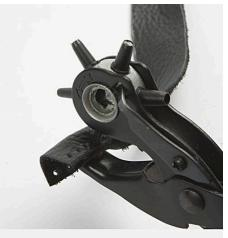
1 Cut a 3cm wide piece of leather in an appropriate length for a bracelet. Fold the piece of leather and punch small holes along the edge with a pair of revolving punch pliers.
