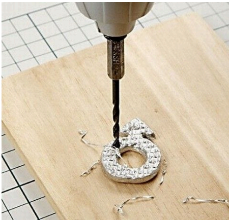
17 Holes are easily drilled in the pewter.
