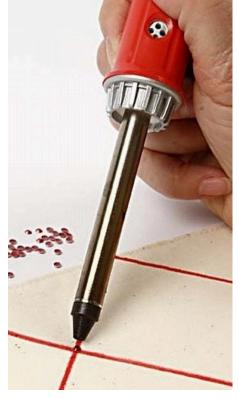
**3** Glue rhinestones onto every intersection with a Hot Fix Applicator. How: Pick up the rhinestones by holding your finger over the hole on the shaft. Move your finger when the tip is pressed down onto the material. The rhinestone is fixed securely.
