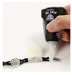
**6.** The plait is held together with a piece of tape whilst gluing the end into an end cap.
