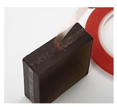
**4** Attach special double-sided adhesive tape along the edge of the lid.
