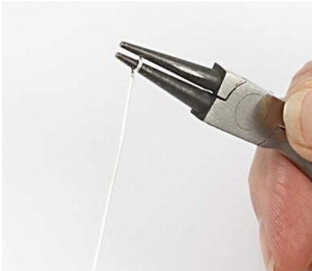
8. On a piece of 0.8mm silver-plated wire, twist to form a loop.
