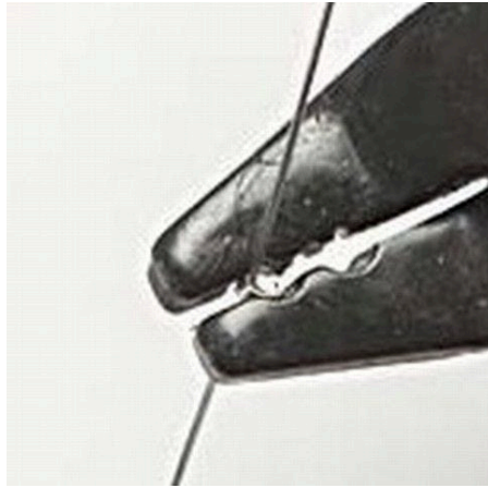
17. With the outer tips of the pliers, gather the bow to make a round bead.
