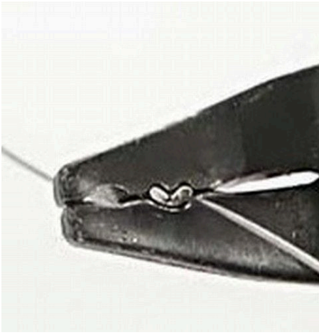
16. The crimp bead is squeezed flat in a bow shape.
