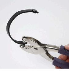
**8.** Squeeze the snap fastener into the hole using the pliers.
