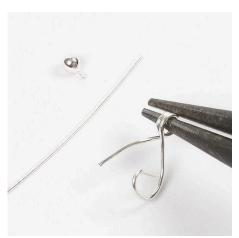
**1.** Cut off the ball of the ball head pin. Twist to form a double loop in the middle of the pin.
