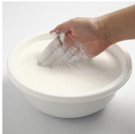
**2.** Stir the mixture - using your hand - until all clumps and bubbles are gone. The consistency should be creamy.
