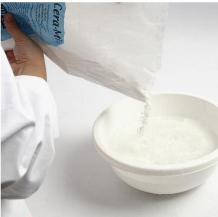
**1.** Pour water into a bowl, and sprinkle plaster into the bowl, forming a small peak above the surface of the water. See the mixing ratio on the packaging of the casting plaster.
