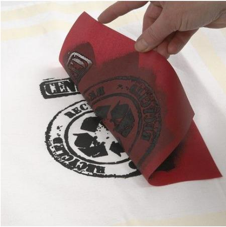
**4.** Remove and wash the screen stencil in lukewarm water immediately. Let the screen stencil print dry. Follow the instructions on the packaging of the paint.
