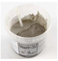
**5** Mix 6 parts of Concrete craft powder to 1 part of water. Put the concrete mixture in a piping bag (disposable) and fill the egg. Let it harden for approx. 24 hours. A TIP! You can make a piping bag from a plain freezing bag by cutting a hole in the corner.
