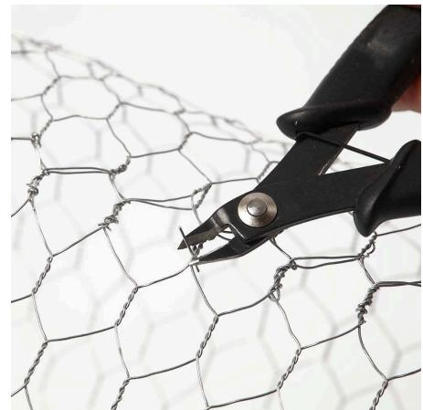
**3** Cut off the excess bits at the ends with flush cutters.
