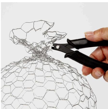
**5** Cut off excess chicken wire netting with flush cutters.
