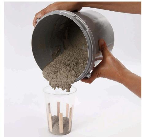
**3** Pour the concrete mixture into the mould and leave for approx. 5 min. NB! Unlike papier-mâché moulds, it is not necessary to coat this mould with cooking oil prior to casting. You may choose to do so, in order to easily release the moulded shape when dry.
