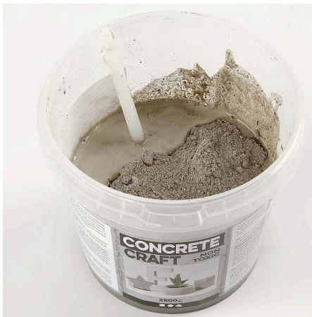
**2** Concrete mixture: Mix 6 parts of Concrete Craft powder to 1 part of water. Mix well and leave for approx. 2 min.
