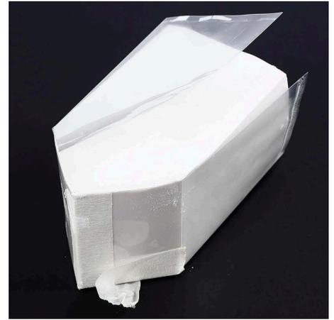
**6** Cut the masking tape and release the moulded shape. Wash the folding mould so that it can be reused.
