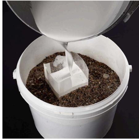
**5** Pour sand into a bucket (for stabilizing the mould during the casting process). Place the mould in the sand and pour the plaster compound into the mould. Tap the sides of the bucket to reduce air bubbles. Leave to set.
