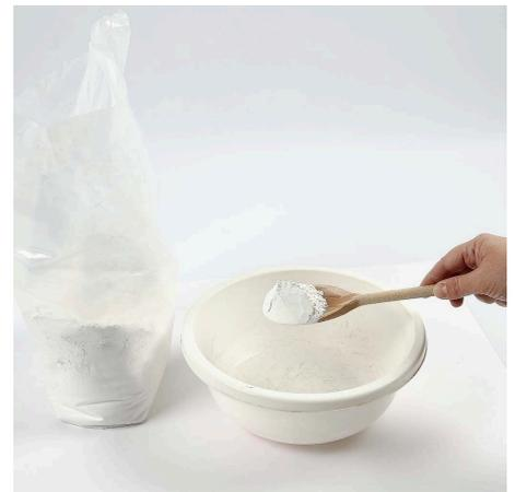
**3** Calculate the mixing ratio (follow the instructions on the packaging) and pour the plaster compound into a bowl.
