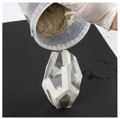
**2** Mix Concrete Craft and water according to instructions on the bucket and pour the mixture into the mould. A TIP: You may use plaster as an alternative.
