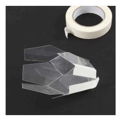
**1** Folding mould: Fold the thin plastic sheet along the scored lines. Seal the joints together with masking tape.
