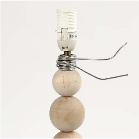
**13** Finish with the lamp socket which is connected to the wire and then secured by twisting it onto the stand, using the loose bonsai wire ends.
