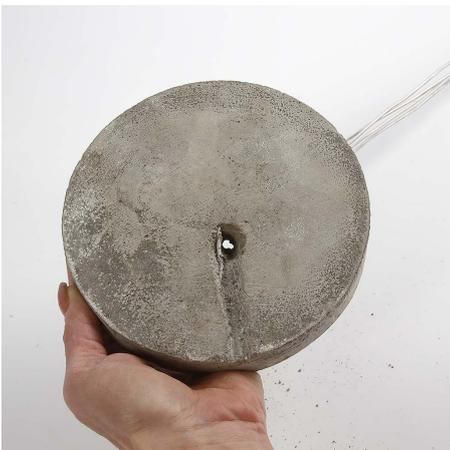
**10** Remove the tape and the small piece of wire that was used in the casting.
