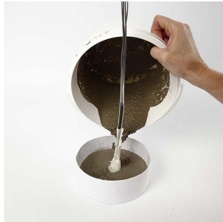
**8** Mix the concrete powder with water following the instructions on the packaging. Pour the liquid concrete into the mould as illustrated. Leave to dry for 24 hours.
