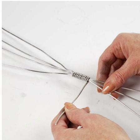
**2** Assemble the four wires by twisting in the middle with one of the four wires, twisting it around itself and the others.
