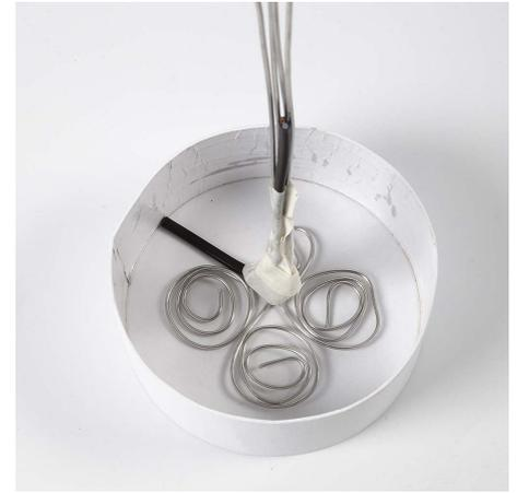
**6** Attach a piece of wire (only to be used for casting) onto the stand using masking tape. Place the stand inside the mould as illustrated.
