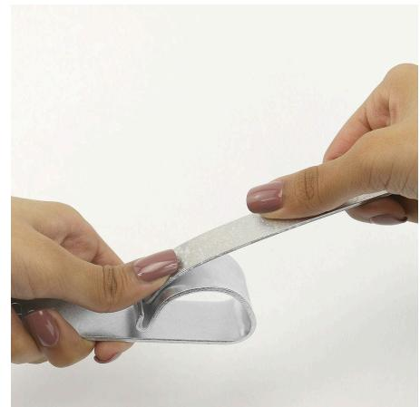
**3** Use the bracelet bending bar to bend the metal band into a cuff shape. Place one end of the metal band into the bending bar face-up. Hold the end securely with your thumb and index finger. Bend the metal band around the bending bar.
