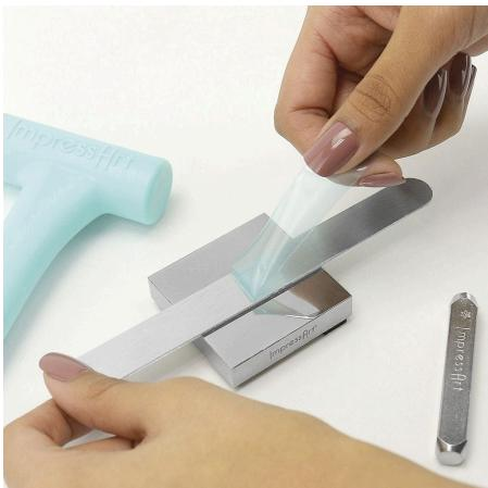
**1** Remove the plastic covering from one side of the metal band and place the metal band on the steel stamping block.
