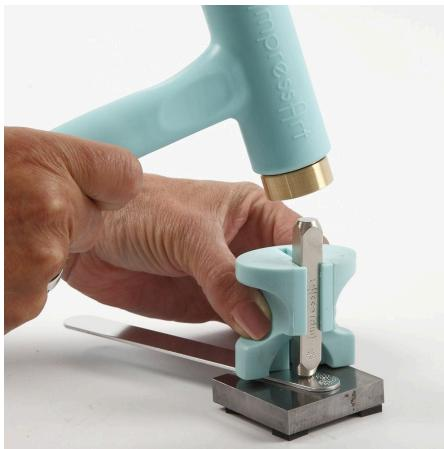
**2** Place the design stamp vertically in the Simple Strike Jig with your chosen design facing the metal band and the Impress Art logo facing you. Strike the embossing stamp once with medium force using the metal stamping hammer. Repeat until the entire metal band is textured.
