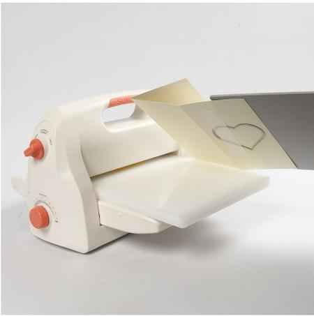
**4** Place the card with the die and the cutting mat inside the die-cutting machine on top of the platform (the thick plate). Now roll the layers through the die-cutting machine.
