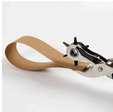
**2** Make holes in the faux leather paper for the hook's screws.
