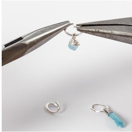
**5** Attach the pendant onto the chain using round jump rings. Close the round jump ring by twisting the two ends together using two pliers.
