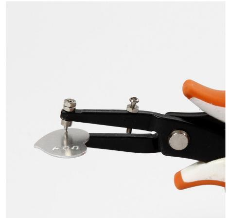
**3** Make a hole in the heart with ImpressArt hole punch pliers.
