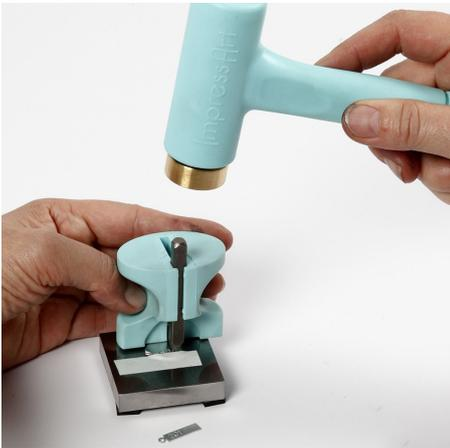
**1** Attach the tag onto the stamping block using stamp straight tape. Attach tape onto the jewellery tag, marking the line. Strike the embossing stamp to write the text.
