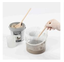
1 Measure the water by putting together two moulds with water inbetween. Pour the water into a transparent bucket and draw a line on the bucket with a marker. Mix concrete and water according to the recommended ratio indicated on the Concrete Craft bucket.
