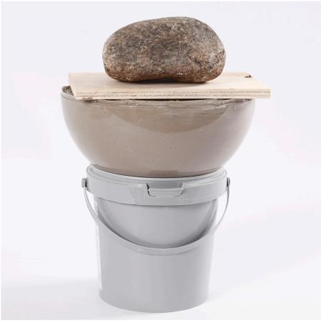
**4** Place a board (or similar) on top and hold it down with a stone or other heavy object. You may moisten the concrete edge in the space between the two moulds and smooth with a finger or a wooden spatula. Alternatively leave it to purposely make a very rough edge. Leave to dry for approx. 2 hours.
