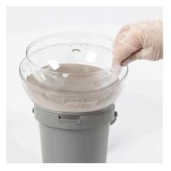
**3** Pour the concrete mixture into the large mould. Press the small mould into the large mould so the edges of both moulds are flush.
