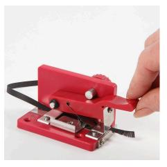
**3** Turn the adjustment dial on the fringer tool to adjust the distance between the cuts. The highest position on the blade gives a wide cut spacing - the lowest position gives a very close spacing.
