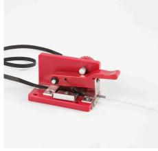
**2** Pull the paper strip forward to the cutting blade.
