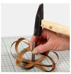
**5** Set the rivet by striking the rivet setting tool with a hammer.
