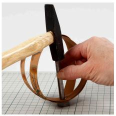
**2** Gather three of the strips and set a rivet by striking the rivet setting tool with a hammer as illustrated in the picture.
