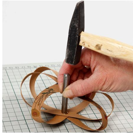
**5** Set the rivet by striking the rivet setting tool with a hammer.
