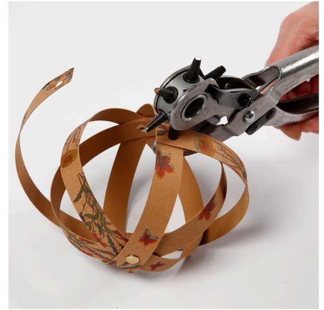
**6** Place the fourth strip around the bauble. Make a hole for a rivet where both ends of the strip meet and set a rivet by striking the rivet setting tool with a hammer.
