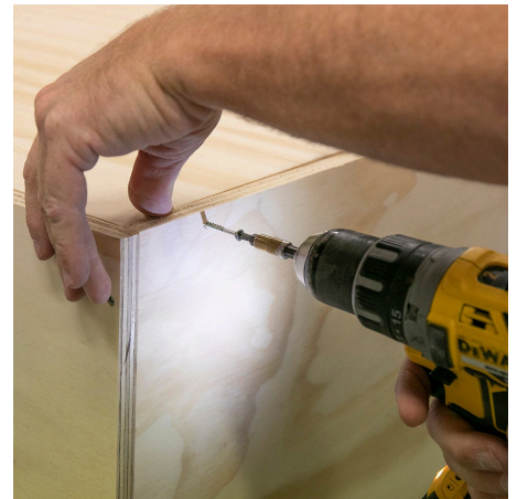
6 Screw on the top board.
