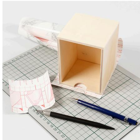
**2** Place the front of the drawers on top of the self-adhesive film. Draw around the outline of the front of the drawer and cut out.
