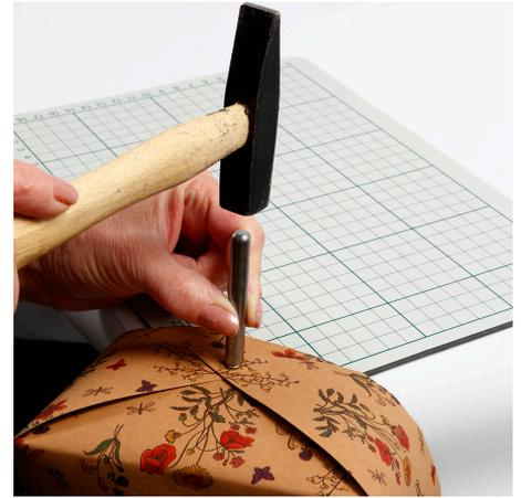
**6** Place the rivets on the concave side of the anvil. Set the rivets by striking the flat end of the rivet setting tool with a hammer.
