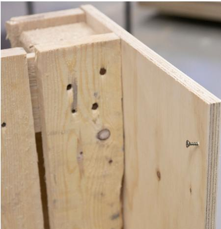
**1** Begin by putting the two half pallets together and then screw on one of the sides. The two short pallet sides measure: 60 x 45 cm and the two long sides measure 83 x 45 cm.
