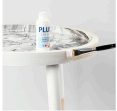
**12** Paint the bottom of the table and screw on the legs. Carefully paint the edges. A TIP: the wooden grain rises when it's being painted. Sand between coats for a smooth finish.
