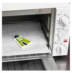
**2** Leave to dry for min. 4 hours and then fix in a household oven at 160°C for 90 min.
