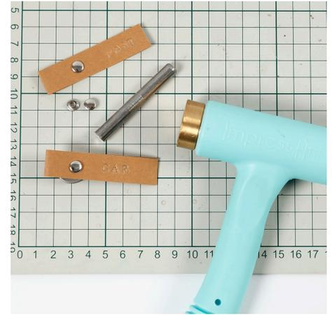
**6** Place the two parts of the rivet through the hole. Use the rivet setting tool and a hammer to set the rivet. Trim the end of the faux leather paper strip. Attach the metal tag and the faux leather paper tag in the keyring.
