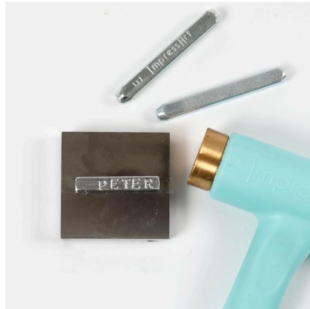
**2** Place the metal tag onto the power tape, preventing it from moving. Hold one letter embossing stamp at a time on the metal tag and strike several times with the metal stamping hammer. Strike firmly with medium force.
