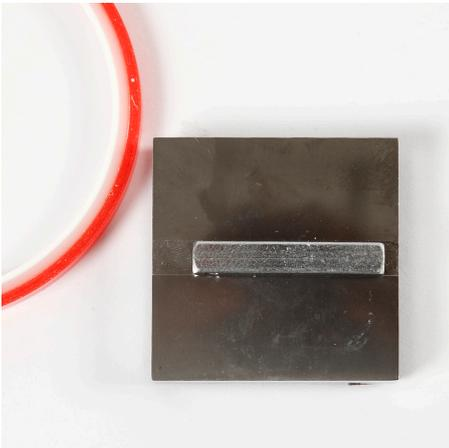
**1** Attach a piece of power tape onto the steel stamping block.
