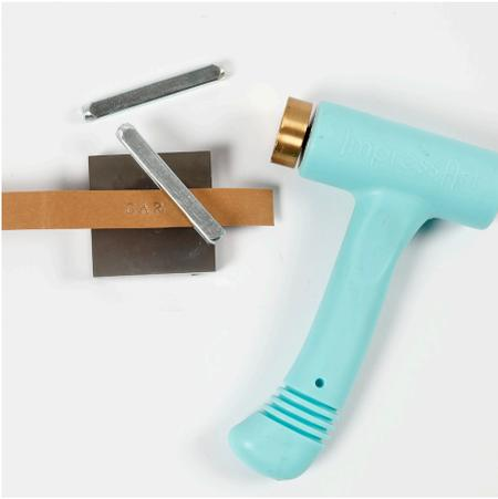
**4** Cut a strip of faux leather paper. Emboss text onto the faux leather paper using the same procedure as when embossing the metal tag. Do not strike too hard with the metal stamping hammer.
