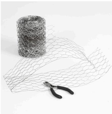
**2** Cut a piece of chicken wire measuring approx. 60-70 cm using side cutters. Fold over.
