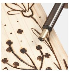
**2** The pyrography tool has different replaceable metal tips.
