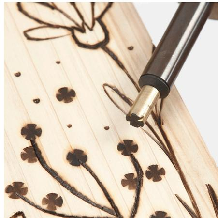
**2** The pyrography tool has different replaceable metal tips.
