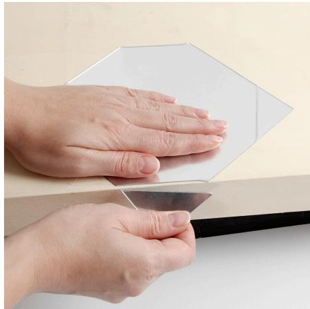
**2** Cut on both sides of the plastic mirror sheet (front and back) and snap off the excess plastic mirror sheet over a table edge. Finish by removing the foil from the front of the plastic mirror sheet.
