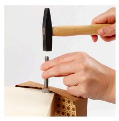
**4** Fold the faux leather paper and secure the joints with a rivet and a rivet setting tool.
