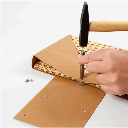
**4** Fold the faux leather paper and assemble with rivets. Place the bottom section of the rivet on the concave side of the anvil, then the faux leather paper on top. Set the rivet by striking the flat end of the rivet setting tool with a hammer as shown in the photo.
