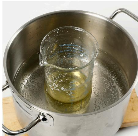
**2** Melt the wax over a water bath at a medium temperature. The melting point of the rapeseed wax is 54-57°C.
