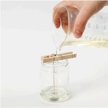
**4** Pour the melted wax into the jam jar. The wax sets after approx. 1.5-2 hours depending on the room temperature and the size of the jar.
