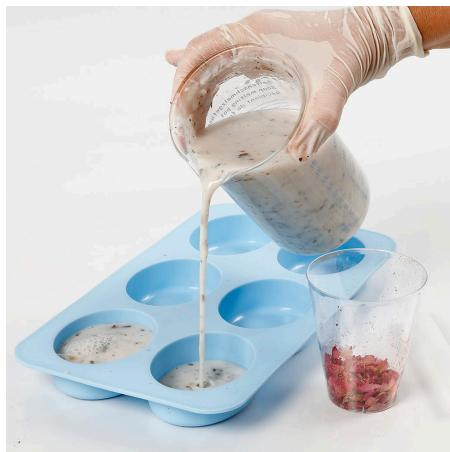
**5** Pour the molten soap into the mould and remove any air bubbles from the surface by spraying with rubbing alcohol.
