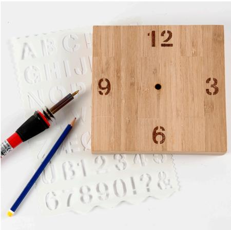
**7** Draw the numbers onto the clock face using a template, then brand the numbers with a pyrography tool. Brand through in the middle of the bamboo veneer which covers the hole for the clock mechanism.
