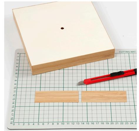
**3** Cut six 3.2 x 19 cm pieces of bamboo veneer to cover the front of the wooden clock box. Cut three of the six pieces in half.
