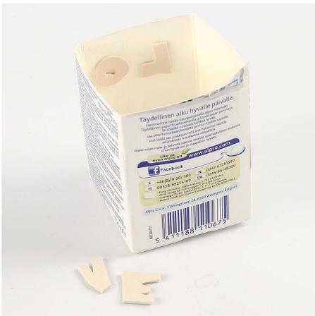
**1** Empty, clean drink cartons are ideal moulds as they are laminated and therefore can withstand wet concrete. Cut off the top bit of the carton. Firmly press shapes and mirrored letters, cut from self-adhesive foam rubber, onto the inside of the carton.
