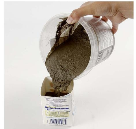
**3** Pour the concrete mixture into the mould and leave for approx. 5 min. NB! Contrary to papier-mâché moulds, it is not necessary to coat this mould with cooking oil prior to casting. You may choose to do so, in order to easily release the moulded shape when dry.
