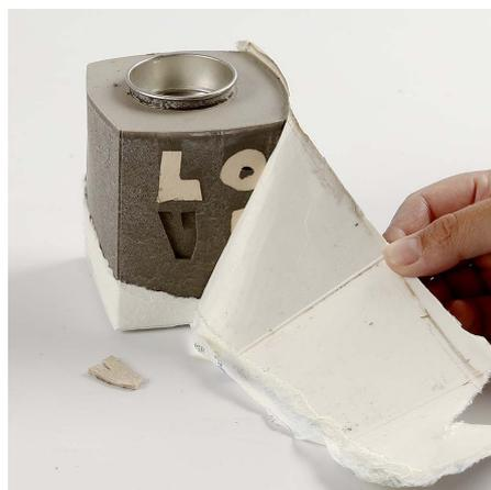
**5** Release the concrete shape from the mould and remove the foam rubber letters/shapes which will break during this procedure.
