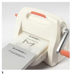
Punch out stars by placing the star die onto the cutting platform with the cutting side facing up. Now place a piece of vellum paper and the cutting mat on top. Make sure that the orange dial on the side is set on Diecut. Run the whole ensemble through the maching in order to punch out a star.
