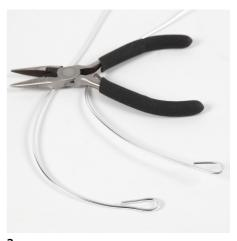
Cut a piece of bonsai wire the same length as the knitted tube. Bend both ends to make a flat loop using pliers.
