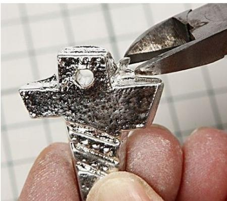
**10** Cut off any pewter sprue with a diagonal cutter.
