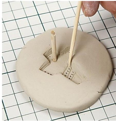
**5** Push a flower stick into the clay where the hole to the o-rings/the cord should be. A pattern can be scratched or pricked into the clay. Holes can also easily be drilled in the pewter after casting.
