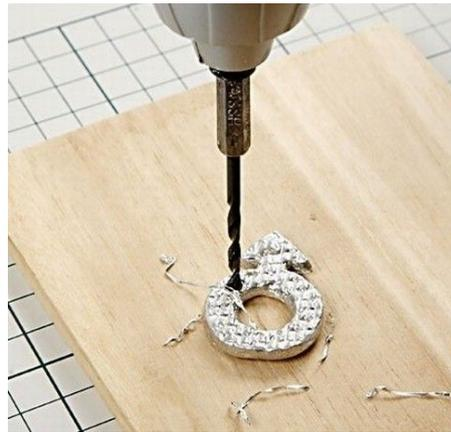
**17** Holes are easily drilled in the pewter.
