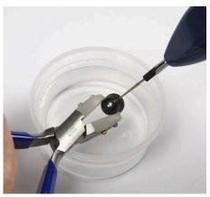
No. 13102 A Bead Reamer This is a special battery operated machine for cleaning and adjusting the bead holes. Hold the bead and the tip of the reamer in some water, and sand off any bumps from the bead hole. The reamer tips are conical and this tool comes with two reamer tips. You will need 2 AA batteries which are not included.
