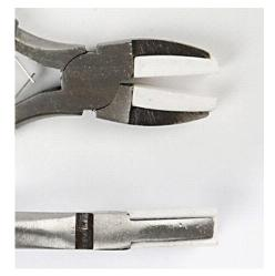
No. 13004 Nylon Jaw Pliers This tool is suitable for squeezing jewellery components without scratching them. When working with soft or shiny jewellery components, this tool is indispensable. It is also suitable for straightening bent metal wire Squeeze hard with the nylon jaw around the wire and pull the wire through the jaw.
